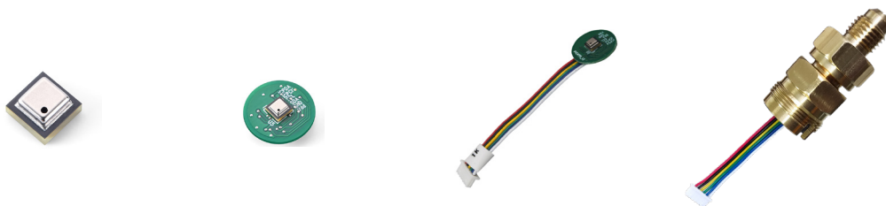
Figure 1a (sensor chip in SMD package), Figure 1b (Pirani vacuum transducer PCB assembly), Figure 1c (transducer + wire harness), Figure 1d (transducer + wire harness packaged in metal fitting)
