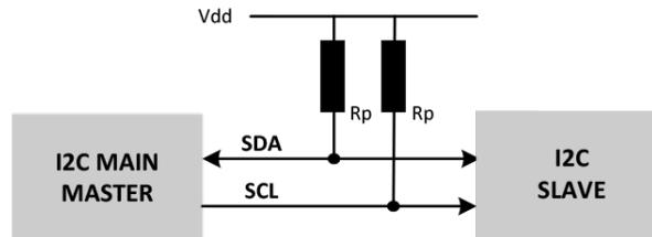
Figure 1: I<sup>2</sup>C master/slave configuration
